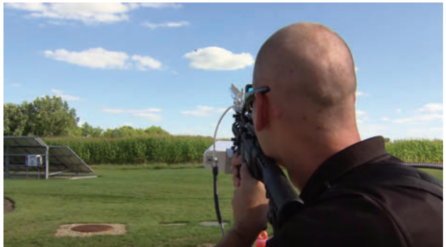
The Battelle DroneDefender system uses RF energy to commandeer encroaching UAVs and lower them safely to the ground. Problems with the U.S. Federal Communications Commission (FCC) has limited its use and deployment.
