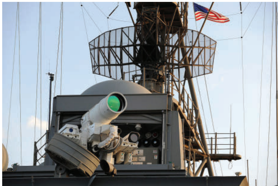
The U.S. Navy AN/SEQ-3 Laser Weapon System (LaWS) can destroy enemy unmanned aircraft, as well as other airborne threats. It was installed on USS Ponce for field testing in 2014.
